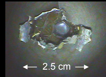
Shuttle radiator damage, 2007
