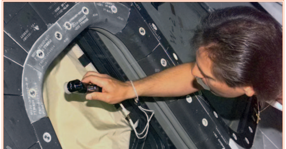
Space Shuttle window being inspected for orbital debris impacts. - Credits: NASA/JSC
